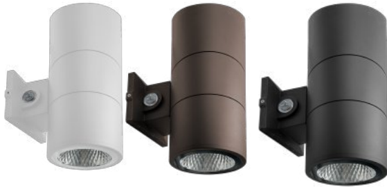
Up/Down LED Light w/ Photocell 4" 12W/16W/20W = 1,260 - 2,100 lm 6" 22W/29W/35W = 2,040 - 3,400 lm Tri-Color (3000K/4000K/5000K) Finishes in Black, White, and Bronze
